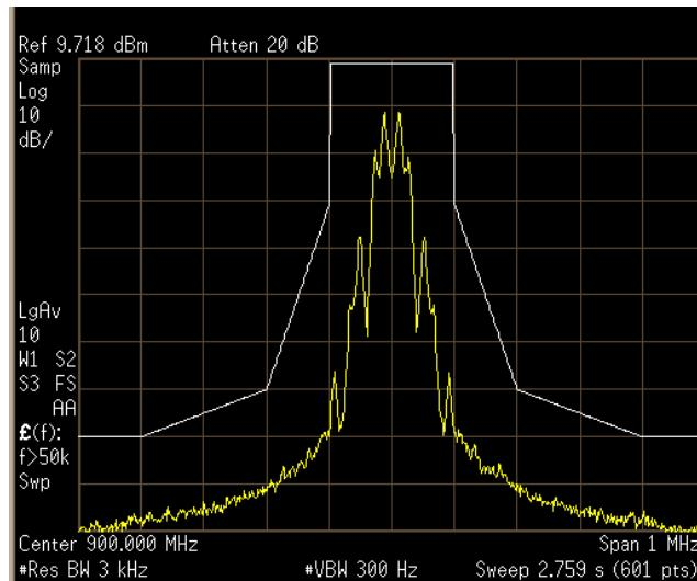
Figure 33: PR-ASK, tari=25μs, X=1.0 turbo mode (+15dBm CW power)
