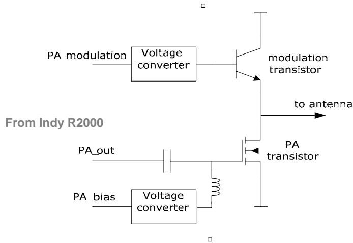
Figure 11: Indy® R2000 Reader Chip Transmit with External PA (DSB ASK)
