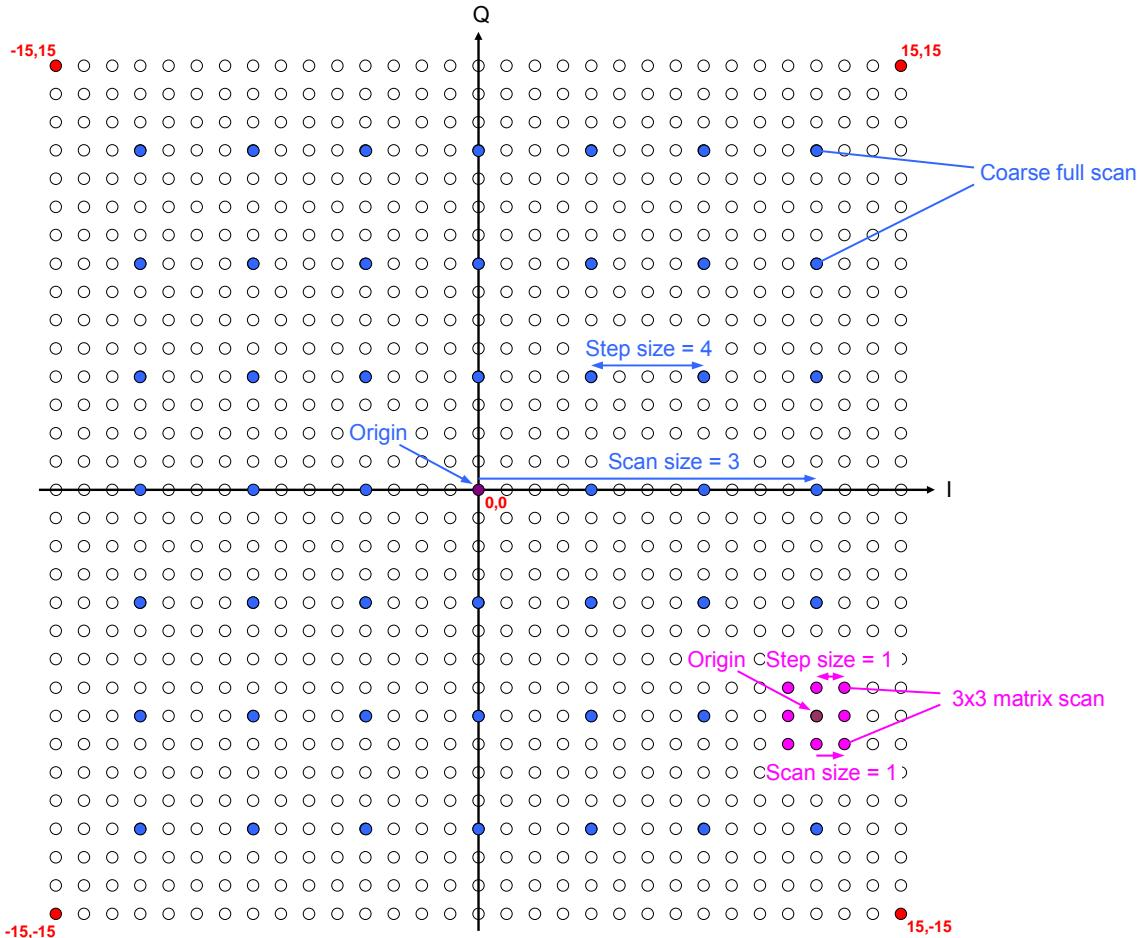
**Figure 8: Self-jammer cancellation grid and calibration examples.**
