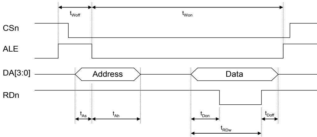
Figure 18: Parallel Interface Read Timing
