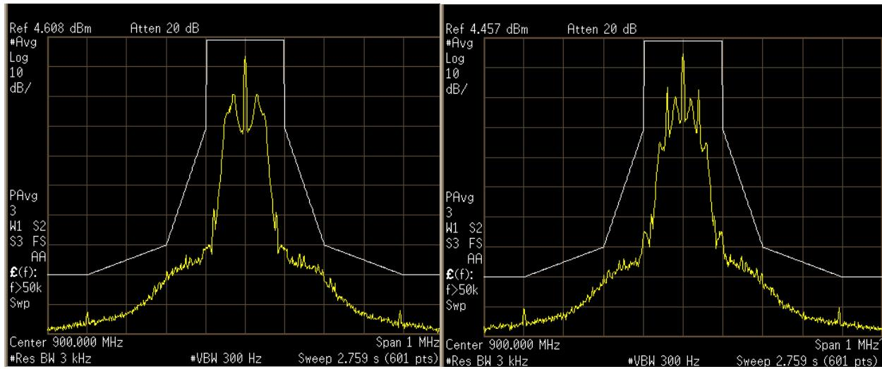
Figure 24: DSB-ASK, tari=25 $\mu$ s, X=0.5 and 1.0
