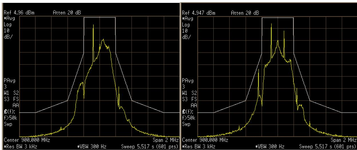
Figure 32: SSB-ASK, tari=6.25μs, X=0.5 and 1.0
