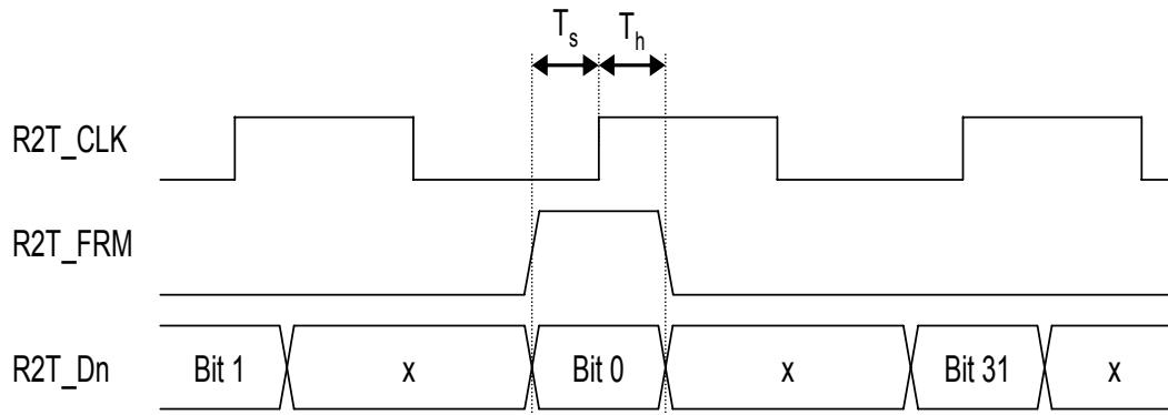
Figure 17: Serial Interface R2T Timing
