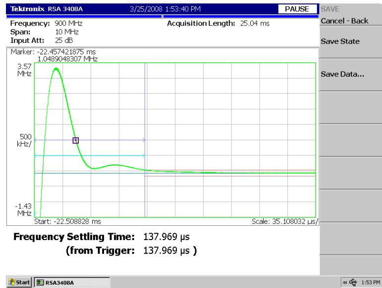
Figure 14: PLL settling time
