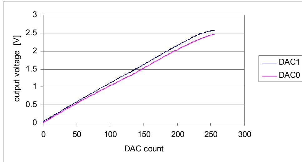
Figure 39: DACs output voltage
