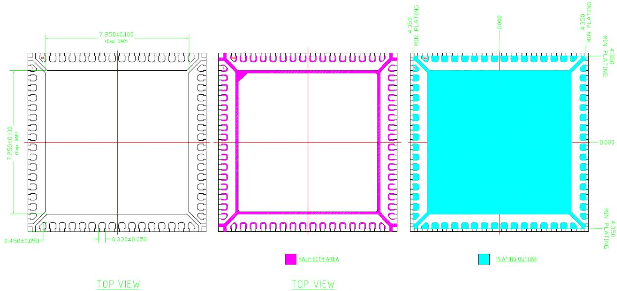
Figure 42: Indy®R2000 reader chip Package Dimensions
