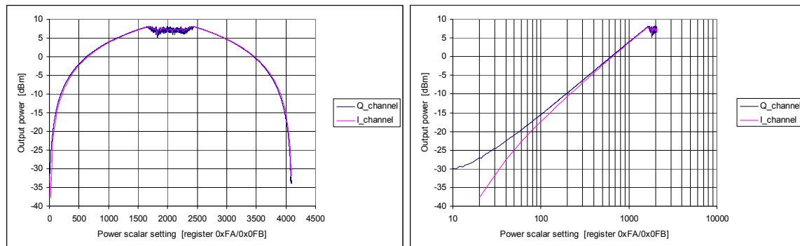
Figure 36: Output power v. scalar state
