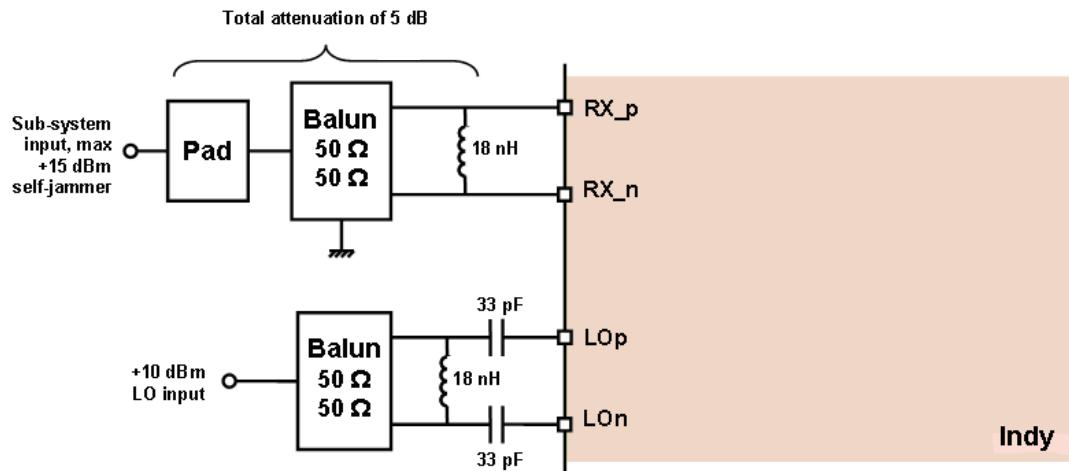
Figure 3: Receiver Front-end External Input Interface Configured to Handle +15 dBm Self-jammer
