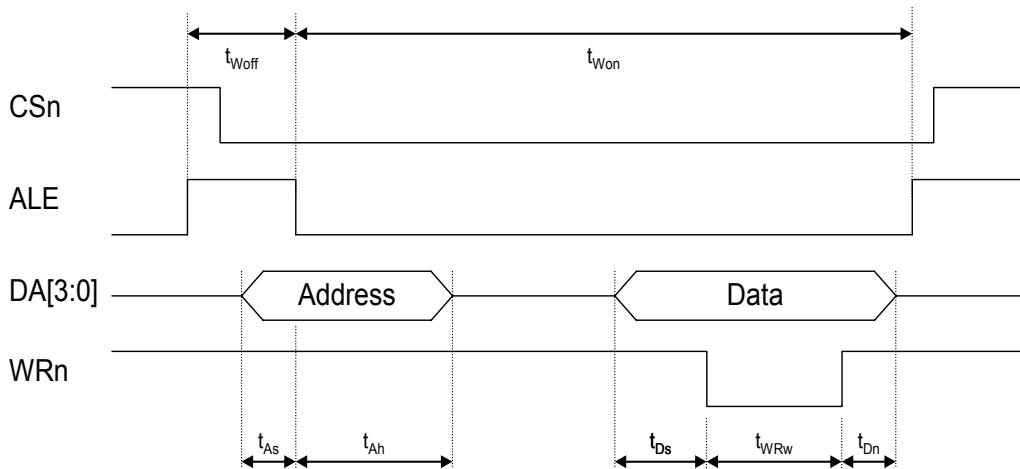
Figure 19: Parallel Interface Write Timing
