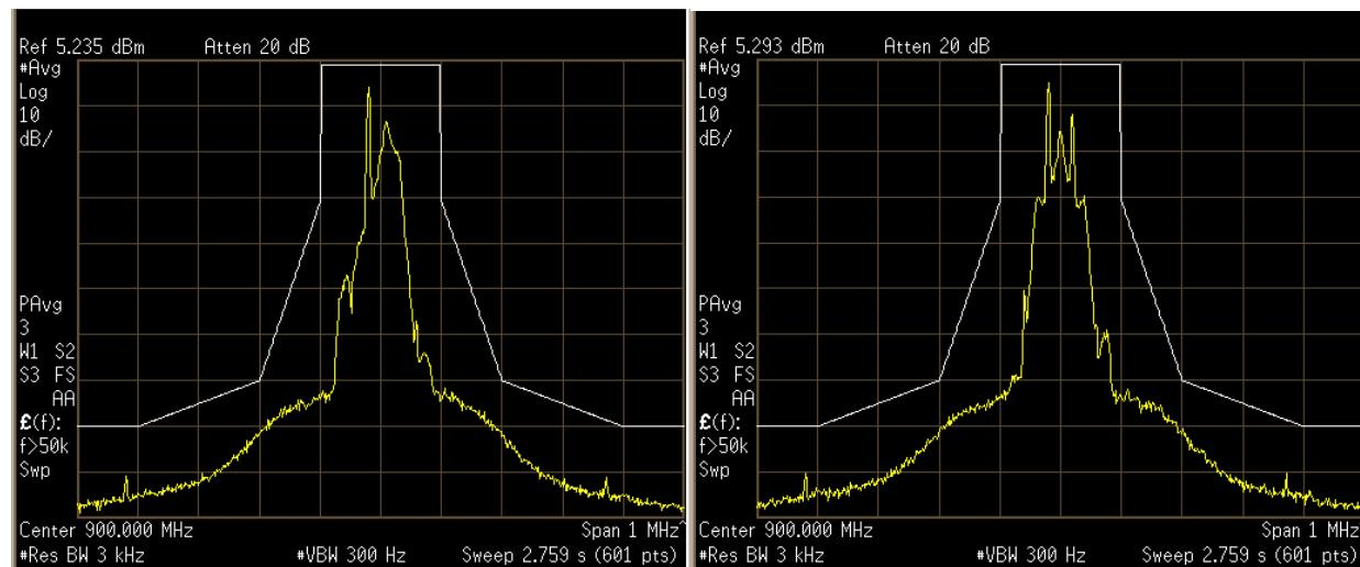
Figure 26: SSB-ASK, tari=25 $\mu$ s, X=0.5 and 1.0
