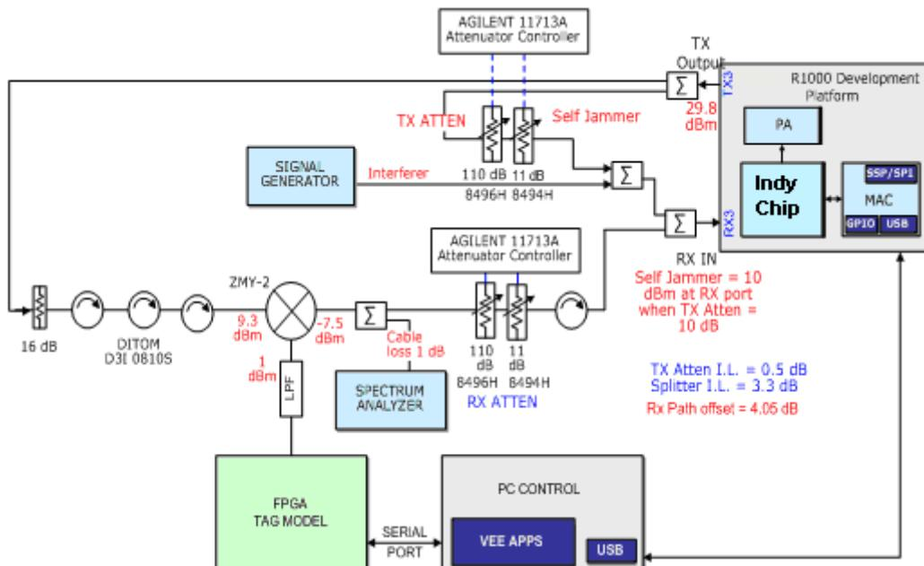
Figure 21: Packet Error Rate Test Setup - Monostatic Configuration
