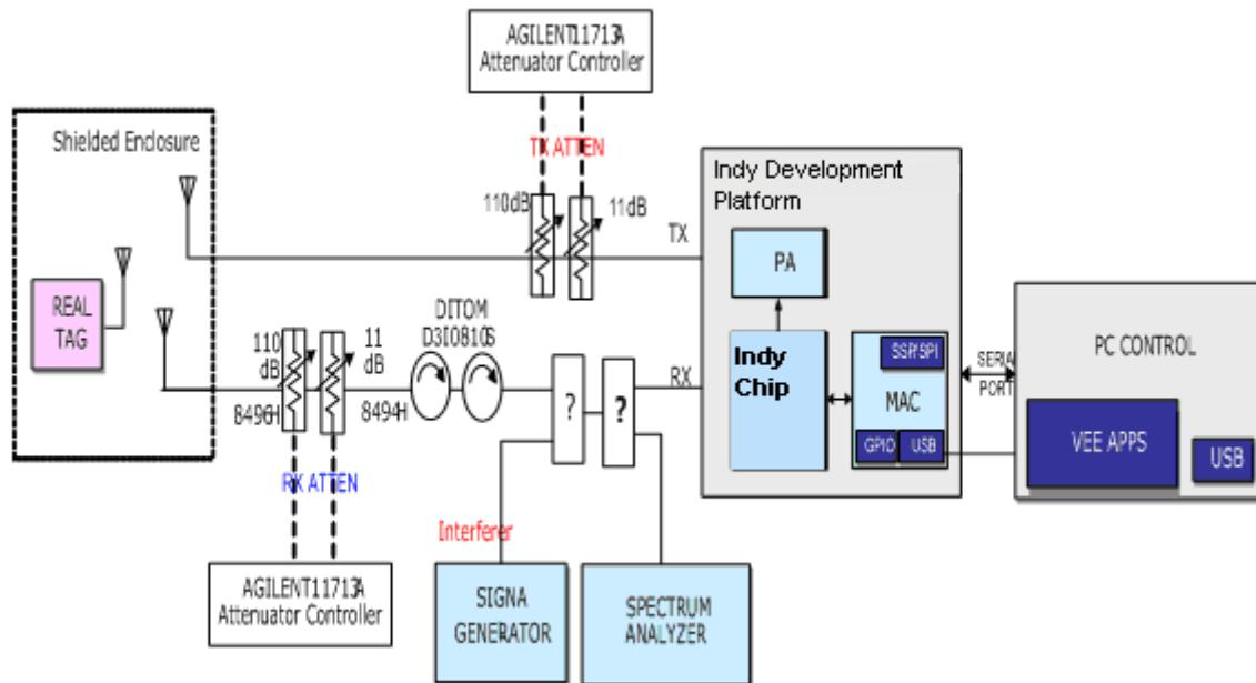
Figure 23: Packet Error Rate Test Setup - Real Tag
