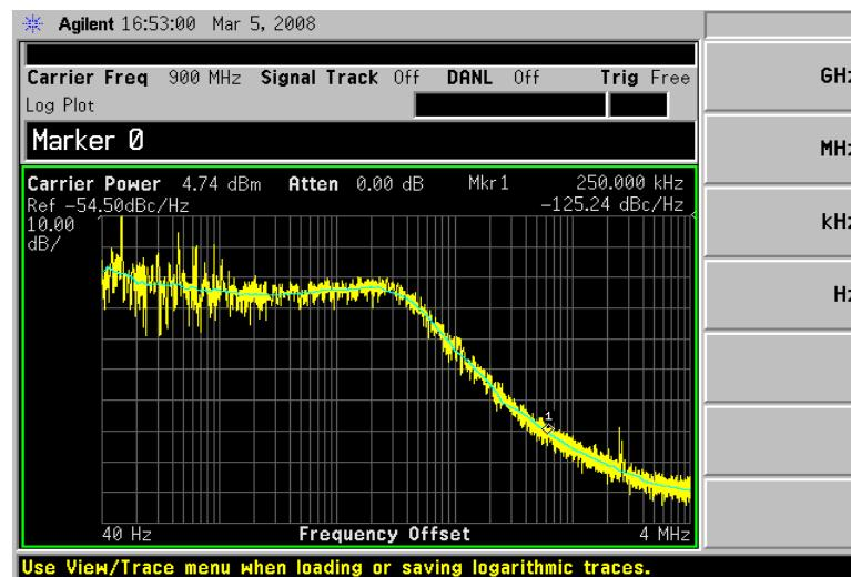
Figure 13: Synthesizer phase noise
