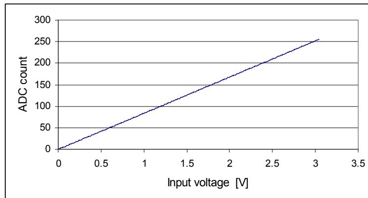
Figure 37: ADC count v. input voltage
