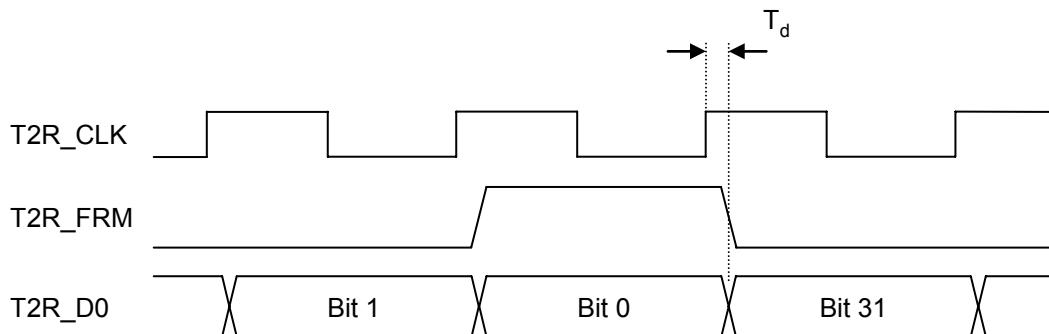
Figure 16: Serial Interface T2R Timing
