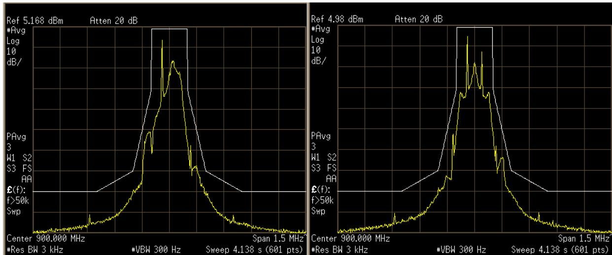
Figure 29: SSB-ASK, tari=12.5 $\mu$ s, X=0.5 and 1.0
