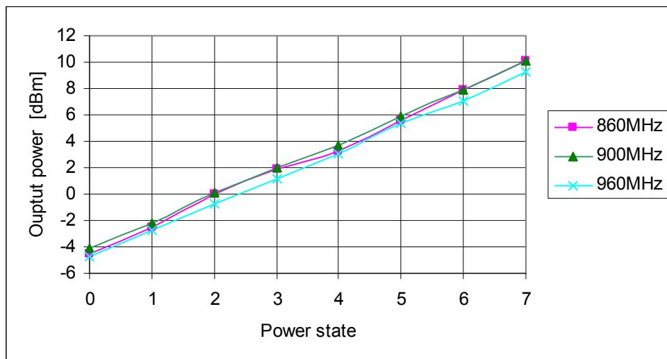
Figure 34: Output power v. analog control state
