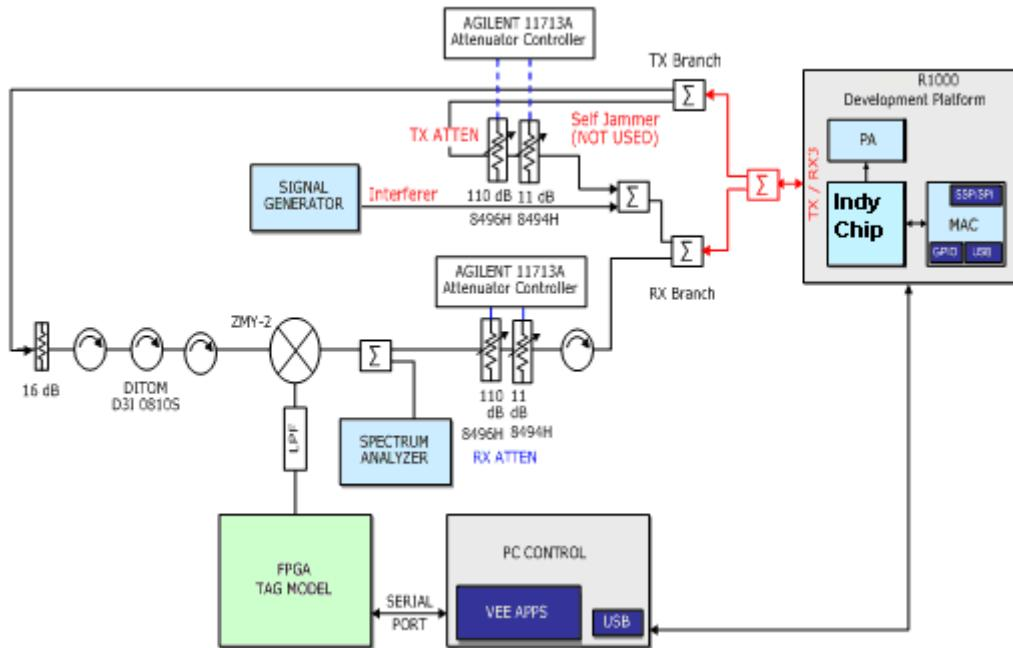
Figure 22: Packet Error Rate Test Setup - Bi-Static Configuration
