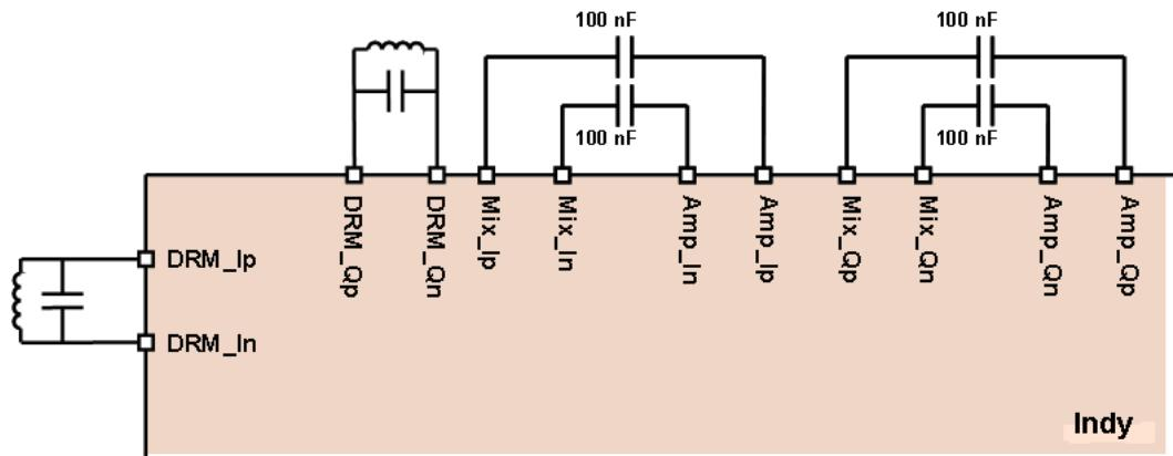
Figure 4: Receiver Front-end External Output Interface, including DRM LC Load of Mixer
