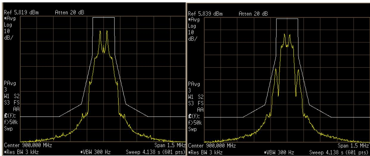
Figure 28: PR-ASK, tari=12.5 $\mu$ s, X=0.5 and 1.0
