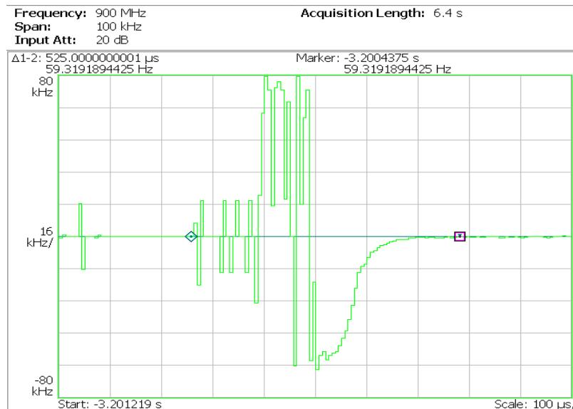
Figure 20: Carrier Settling Time
