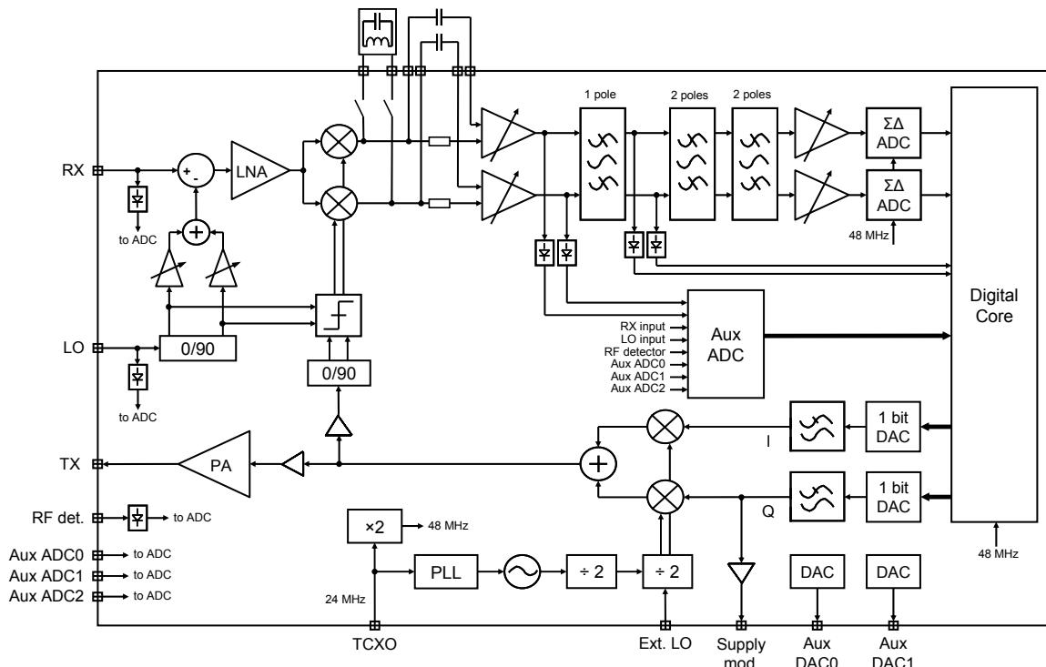
Figure 1: Indy R2000 Reader Chip Top Level RF Block Diagram
