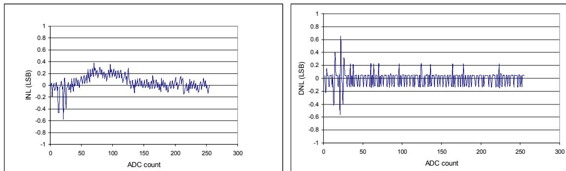
Figure 35: INL and DNL for auxiliary ADC
