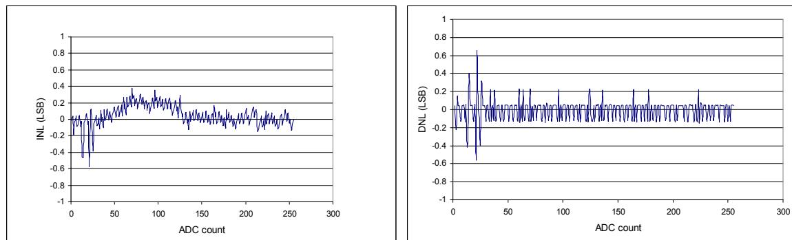
Figure 38: INL and DNL for auxiliary ADC
