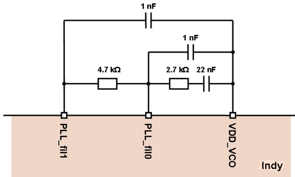
Figure 5: Local Oscillator Input External Interfaces
