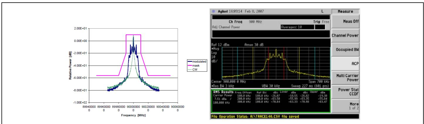
**Figure 28: Indy R1000 Reader Chip Transmit Modulation and Mask for DSB, Tari=25  $\mu$ sec, X=1**
